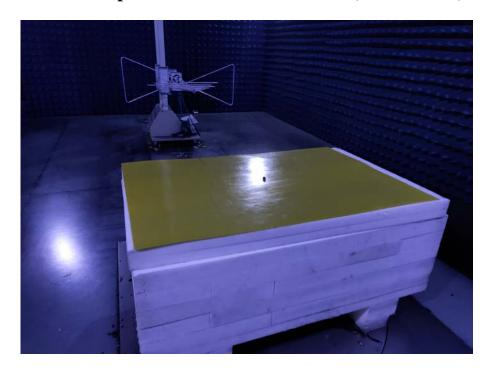
**Radiated Spurious Emissions Test View (Above 1GHz)**
