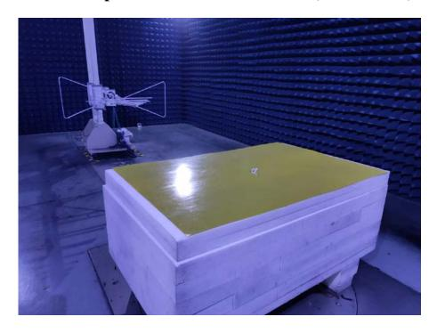
**Radiated Spurious Emissions Test View (Above 1GHz)**
