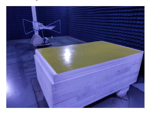
Radiated Spurious Emissions Test View (Above 1GHz)
