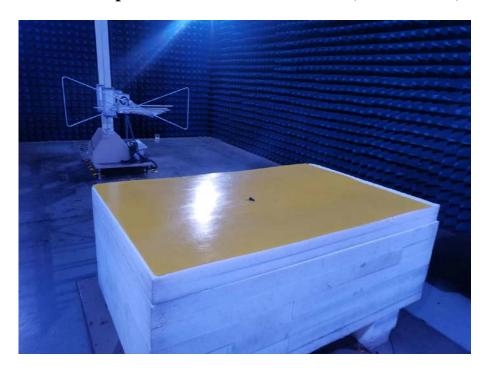
**Radiated Spurious Emissions Test View (Above 1GHz)**
