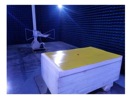
Photo of Radiated Emission Measurement Above 1GHz
