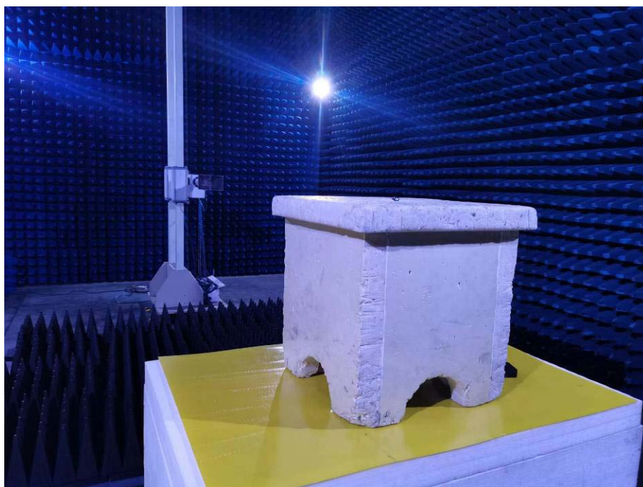
Photo of Radiated Emission Measurement Above 1GHz
