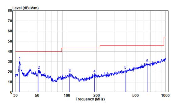
Site : chamber Condition: 3m VERTICAL Model : EP-0664
