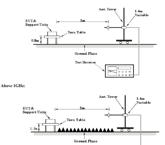
The radiated emission tests were performed in the 3 meters, using the setup accordance with the ANSI C63.10-2013. The specification used was the FCC 15.209 and FCC 15.247 limits.
