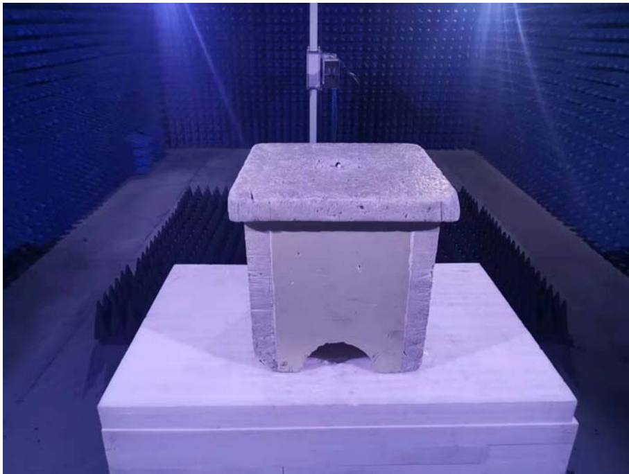
Photo of Radiated Emission Measurement Above 1GHz
