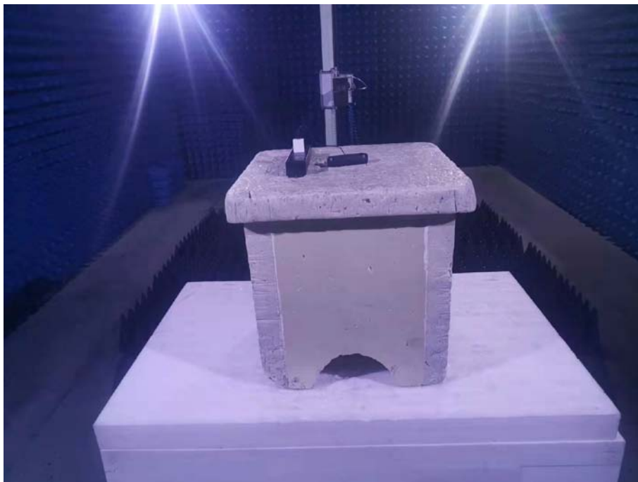
Photo of Radiated Emission Measurement Above 1GHz
