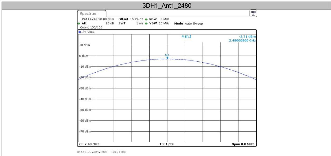
**Appendix C: Carrier frequency separation****Test Result**
