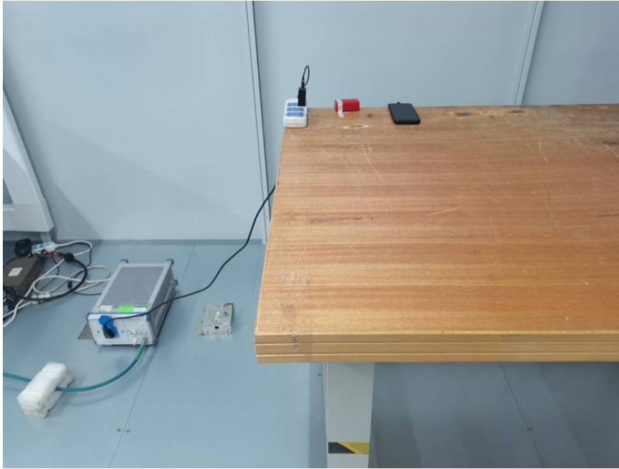
Conducted Emissions - Front View
