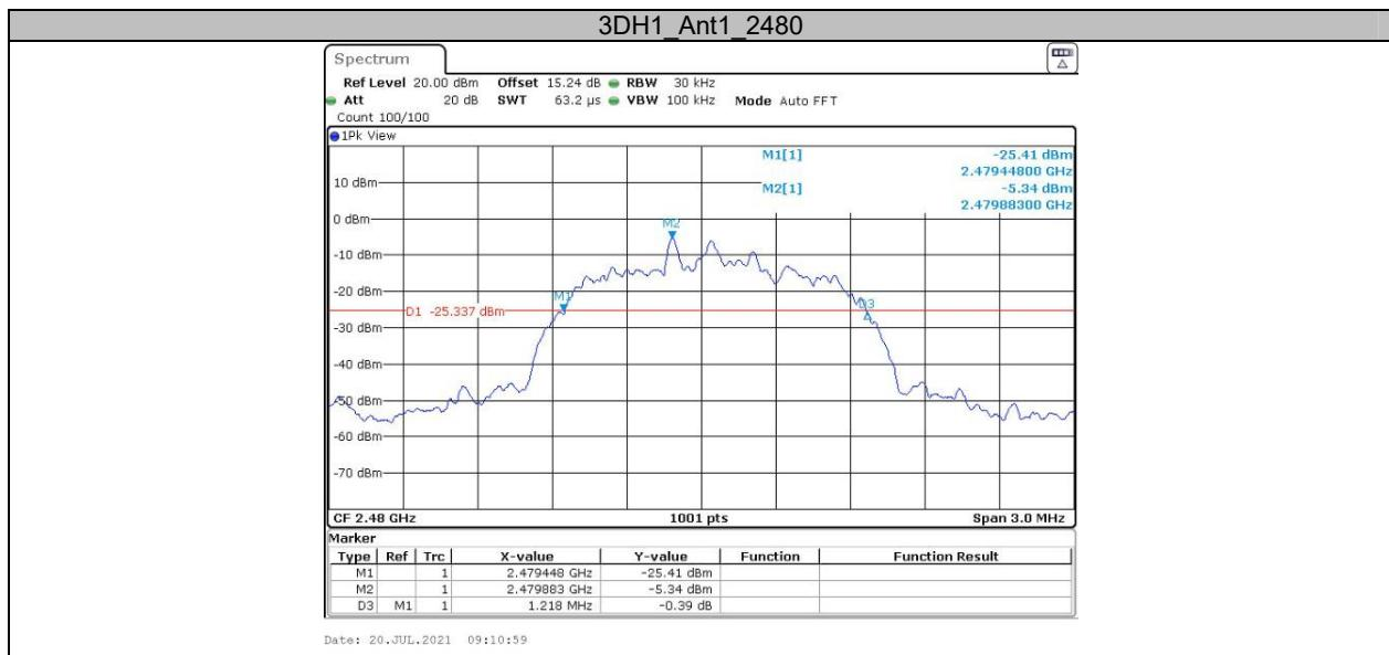
**Appendix B: Occupied Channel Bandwidth****Test Result**
