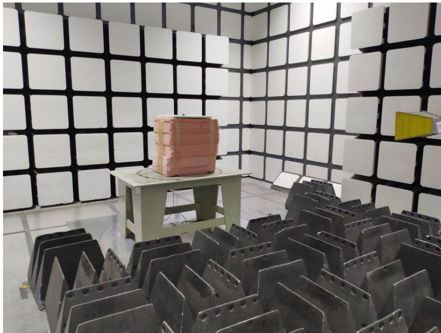
Radiated Emissions View (Above 1 GHz)
