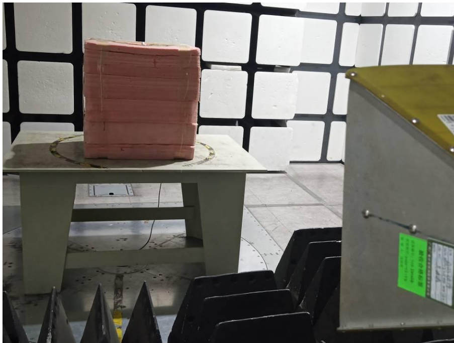
Radiated Emissions View (Above 1 GHz)
