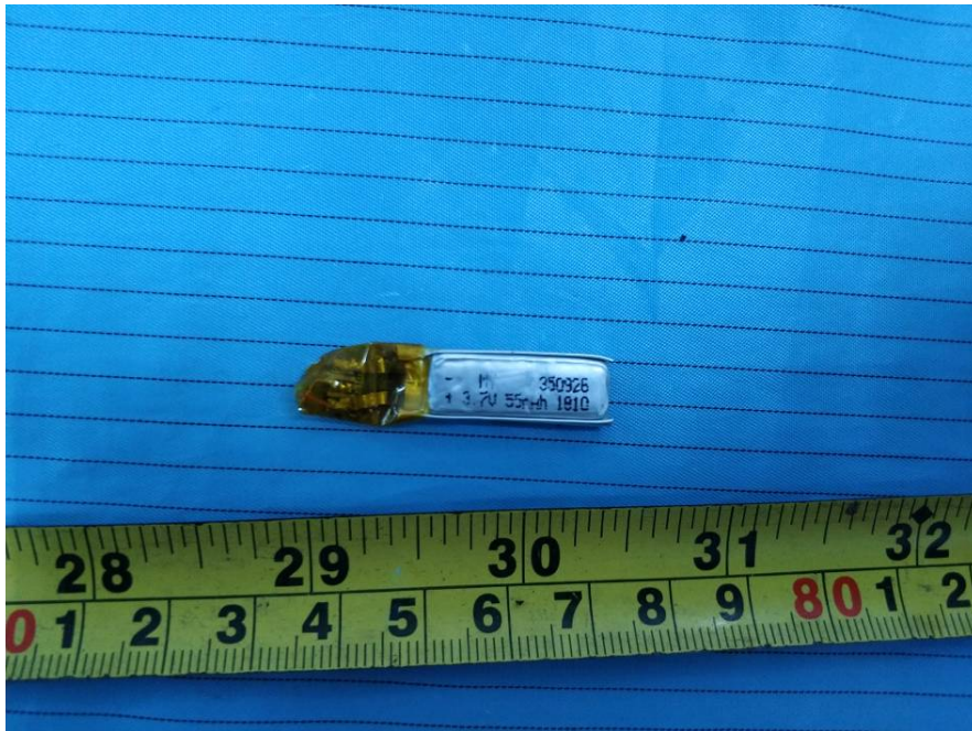
EUT – Battery Front View
