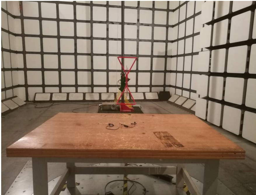
Radiated Emissions View (Below 1 GHz)
