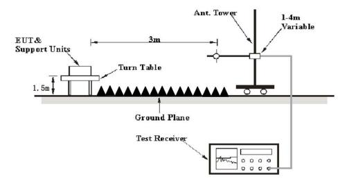
The radiated emission tests were performed in the 3 meters, using the setup accordance with the ANSI C63.10-2013. The specification used was the FCC 15.209, 205 and FCC 15.247 limits.
