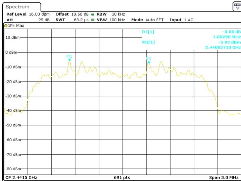
**EDR ( $\pi/4$ -DQPSK): High Channel**
