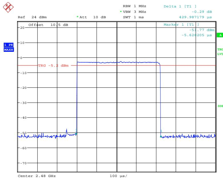
**Pulse time, Low Channel, 2DH3**
