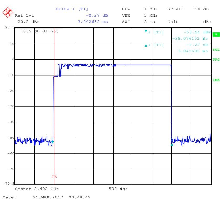
**Pulse time, Middle Channel, 2DH5**
