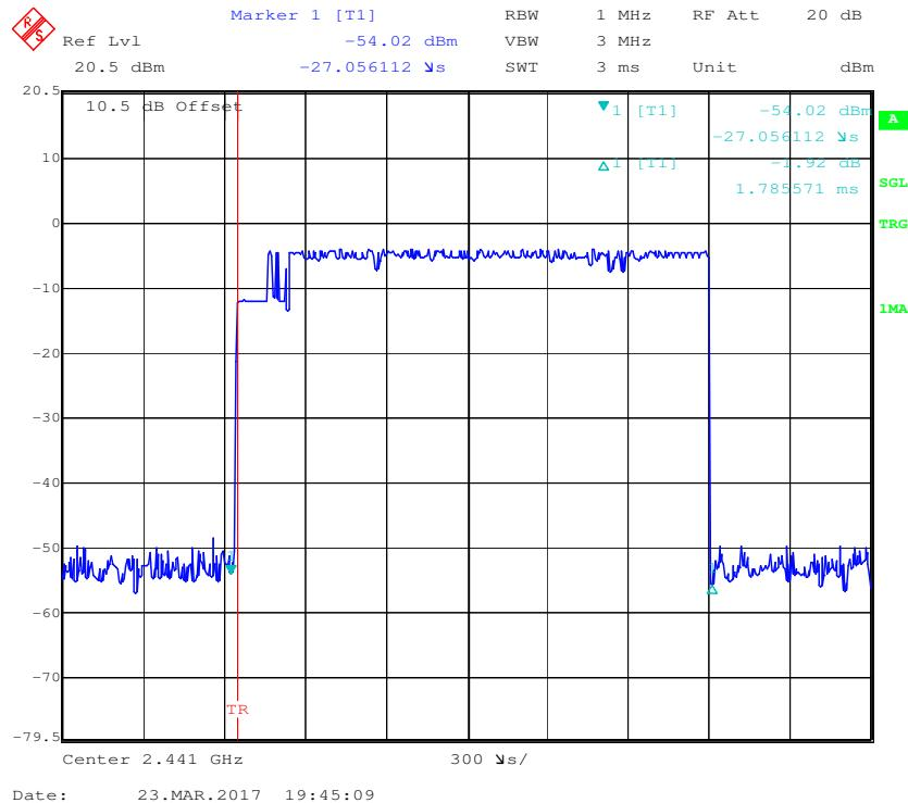
**Pulse time, High Channel, 2DH3**
