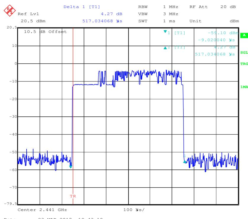
**Pulse time, High Channel, 3DH1**
