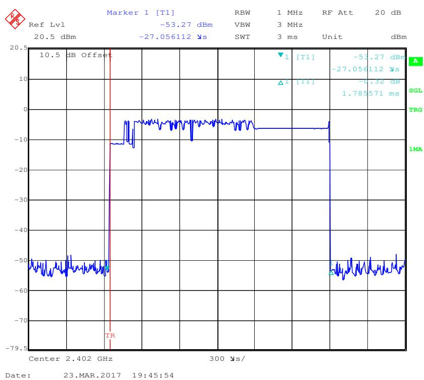
**Pulse time, Middle Channel, 3DH3**
