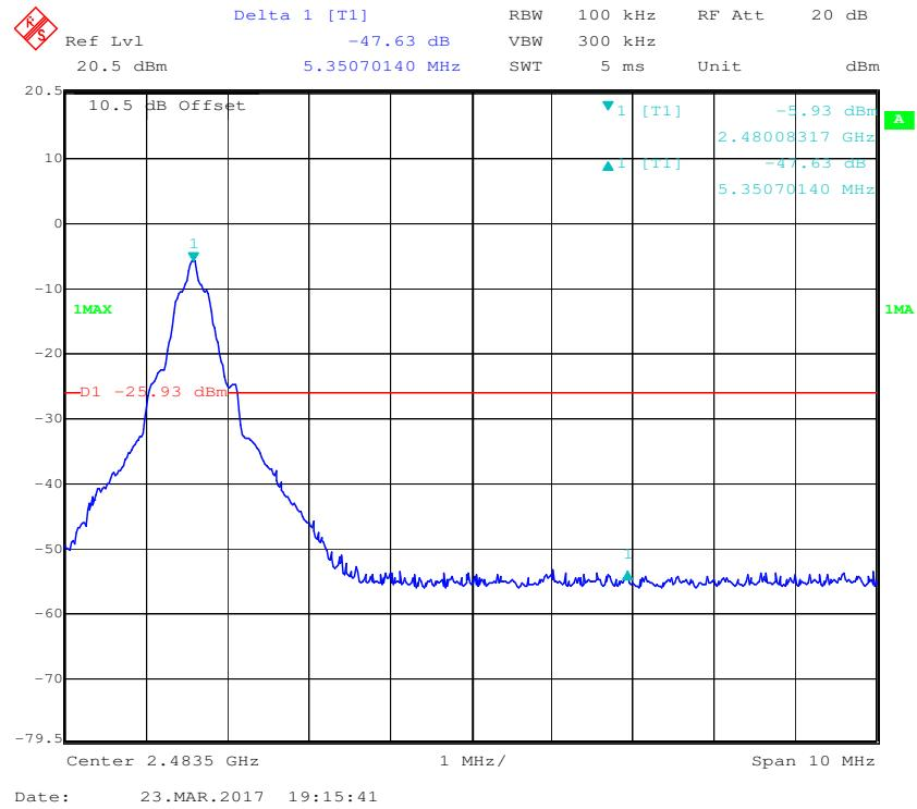
**EDR ( $\pi/4$ -DQPSK): Band Edge-Left Side**
