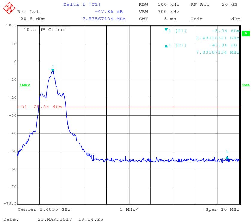
**EDR (8DPSK): Band Edge-Left Side**
