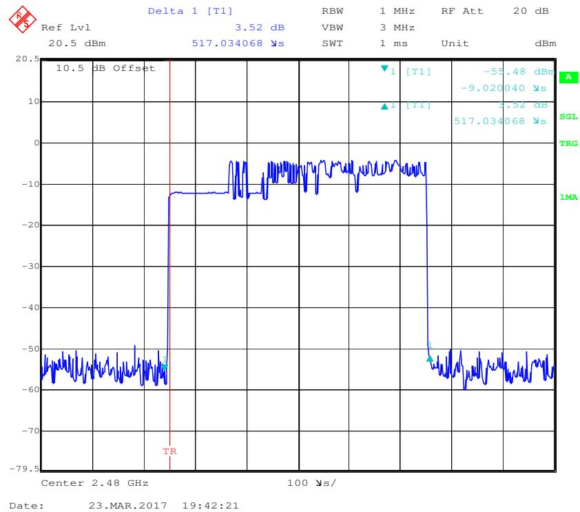
**Pulse time, Low Channel, 2DH3**
