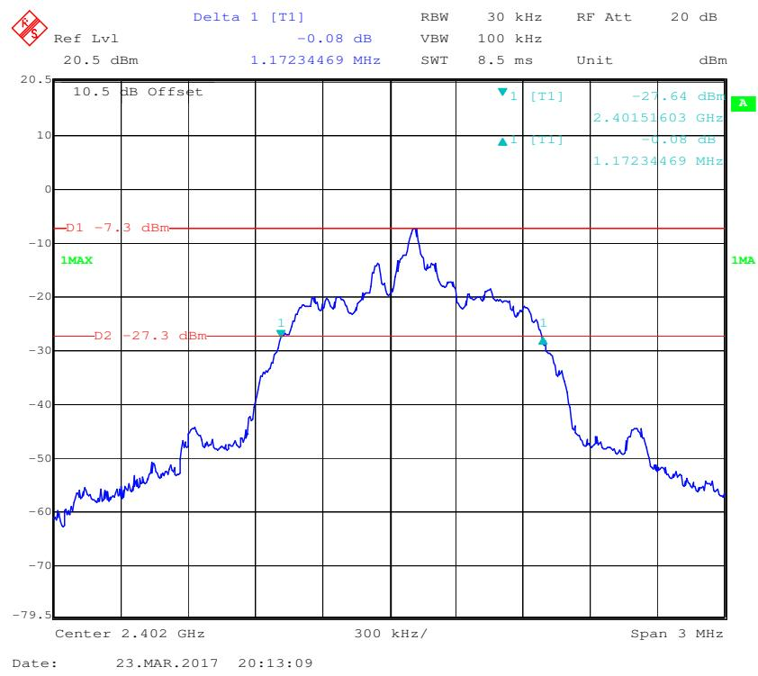
**EDR ( $\pi/4$ -DQPSK): Middle Channel**
