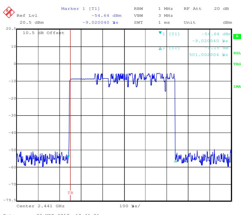
**Pulse time, High Channel, DH1**
