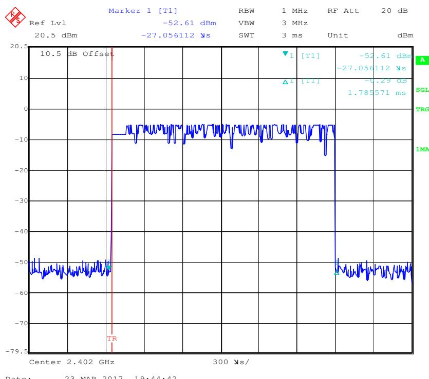
**Pulse time, Middle Channel, DH3**
