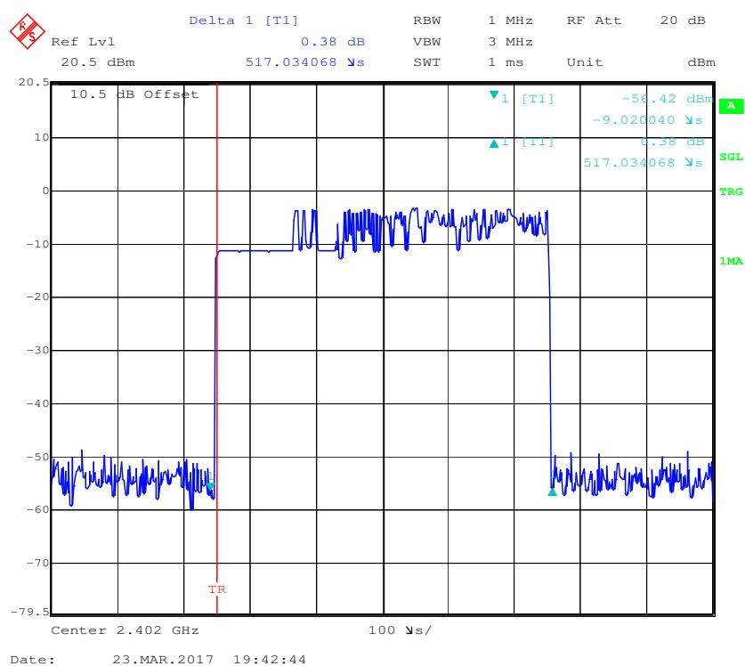
**Pulse time, Middle Channel, 2DH1**
