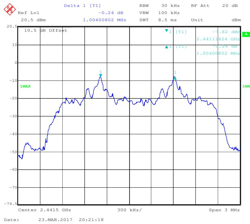
**EDR ( $\pi/4$ -DQPSK): High Channel**
