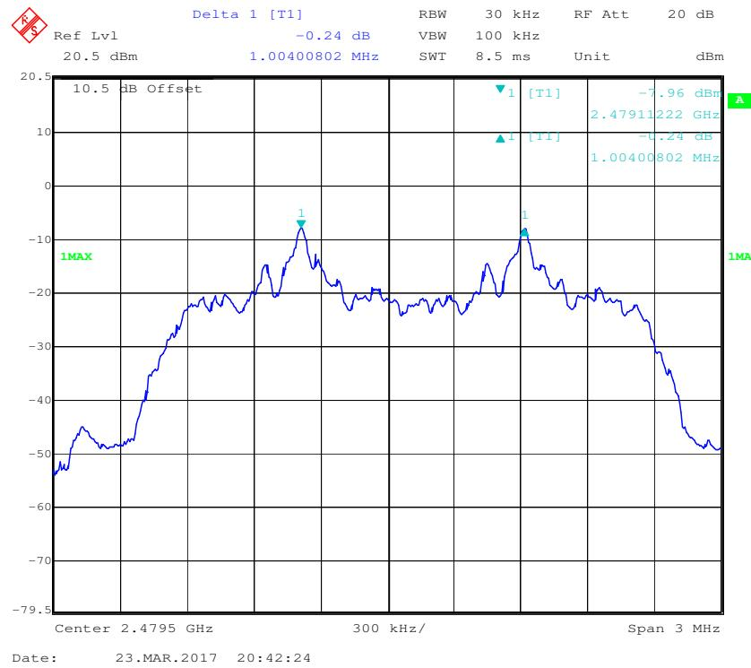
**EDR (8DPSK): Low Channel**
