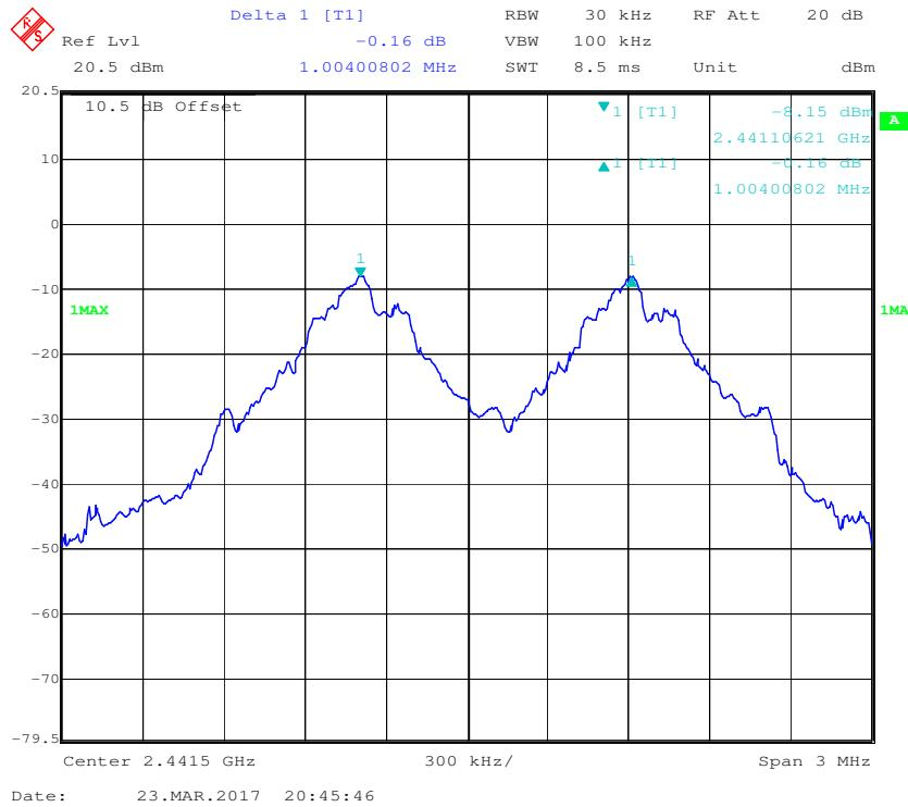
**BDR (GFSK): High Channel**
