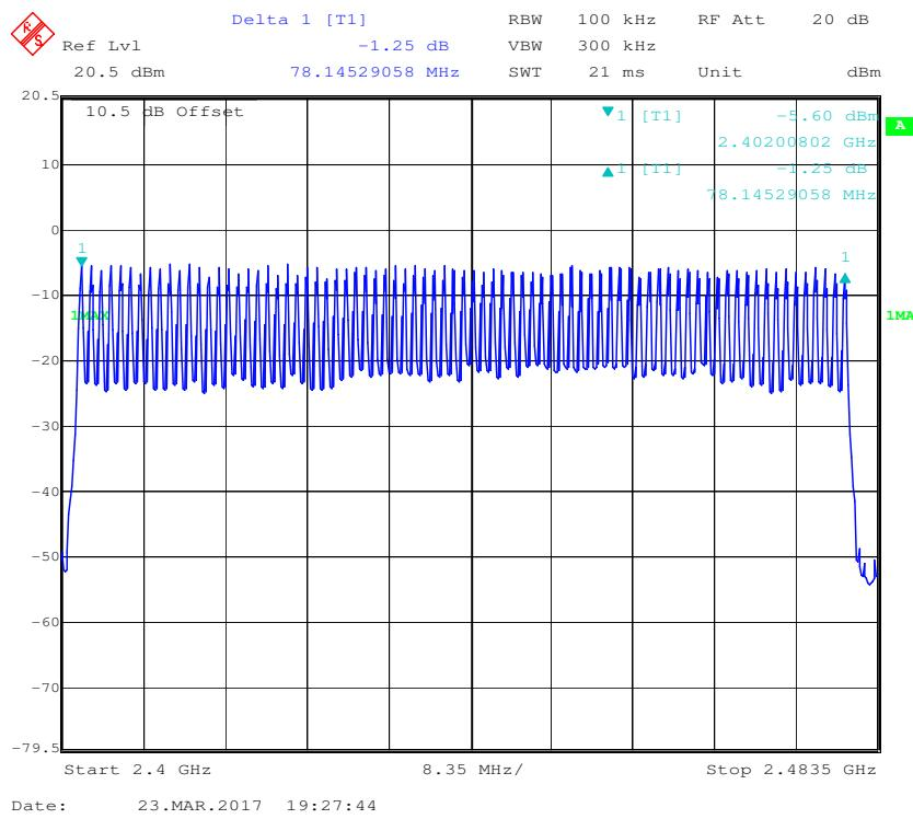
**EDR ( $\pi/4$ -DQPSK): Number of Hopping Channels**
