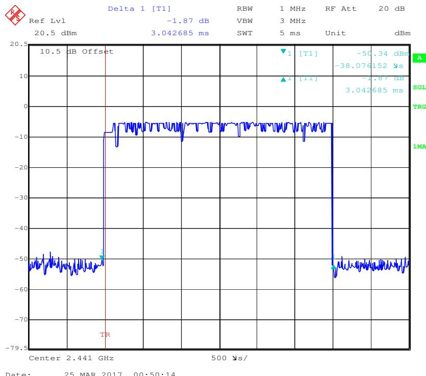
**Pulse time, High Channel, DH5**
