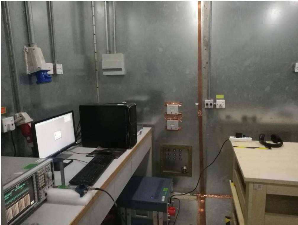
FCC RADIATED EMISSION TEST SETUP
