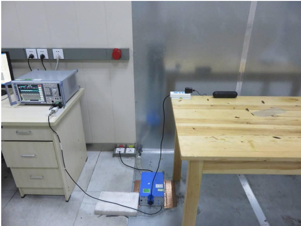
FCC RADIATED EMISSION TEST SETUP
