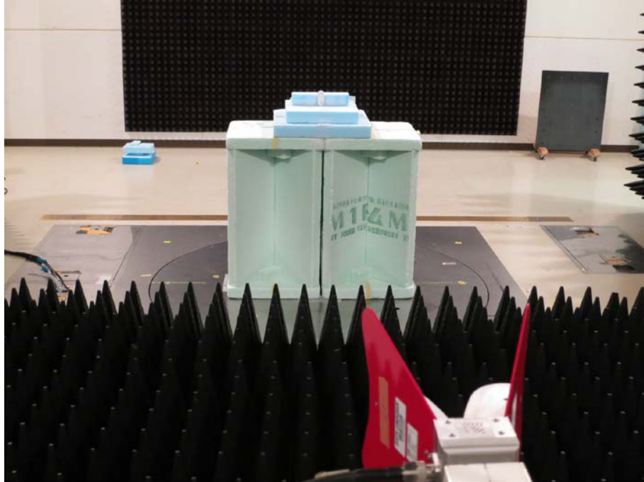
Photo1 Test setup for radiated (above 1GHz)
