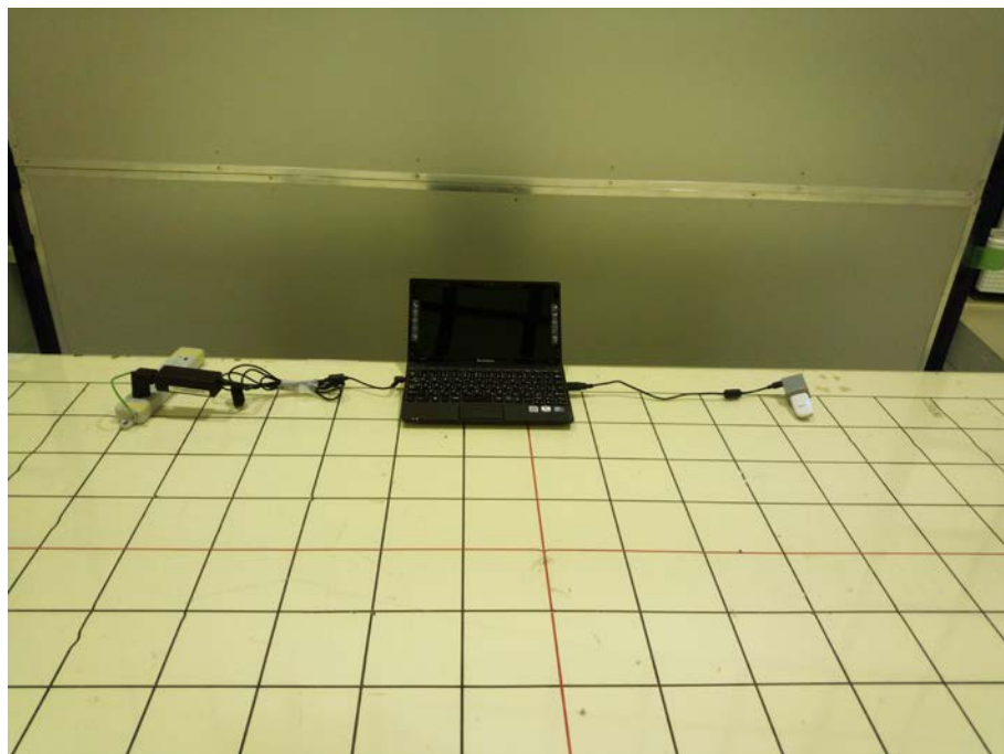
Photo6 Test setup for conducted(AC Line)
