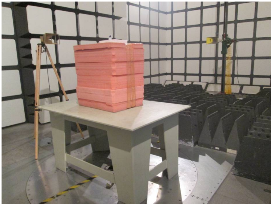
Radiated Emissions Test View (Above 1 GHz)
