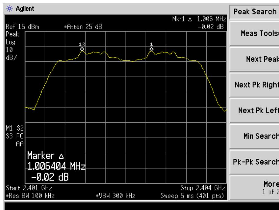
Channel Spacing (Middle CH=1MHz)
