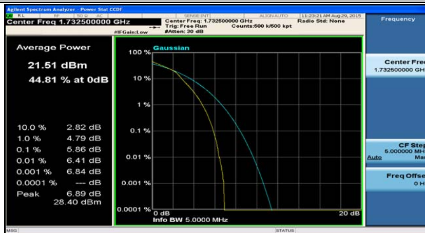
(Channel Bandwidth: 5 MHz)_MCH_16QAM_12RB#6
