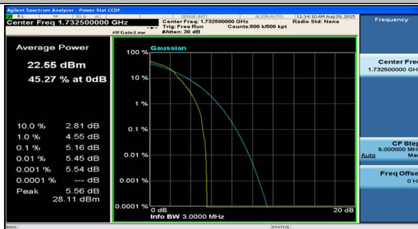
(Channel Bandwidth: 3 MHz)_MCH_16QAM_1RB#7
