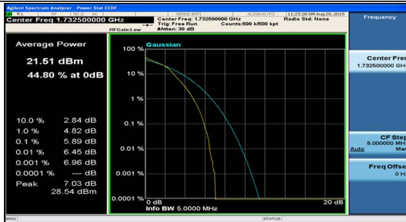
(Channel Bandwidth: 5 MHz)_MCH_16QAM_25RB#0
