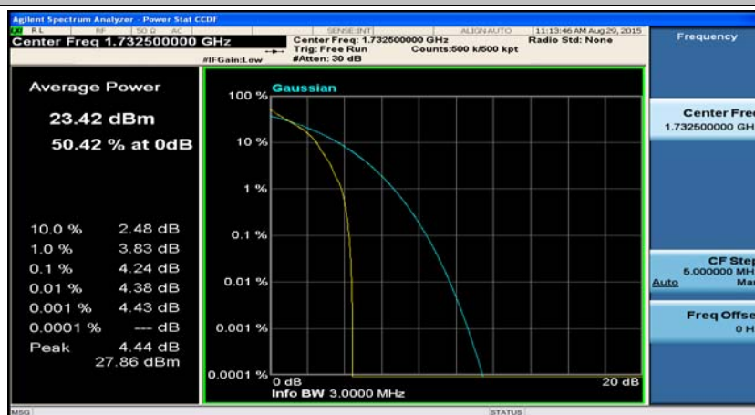
(Channel Bandwidth: 3 MHz)_MCH_QPSK_1RB#7
