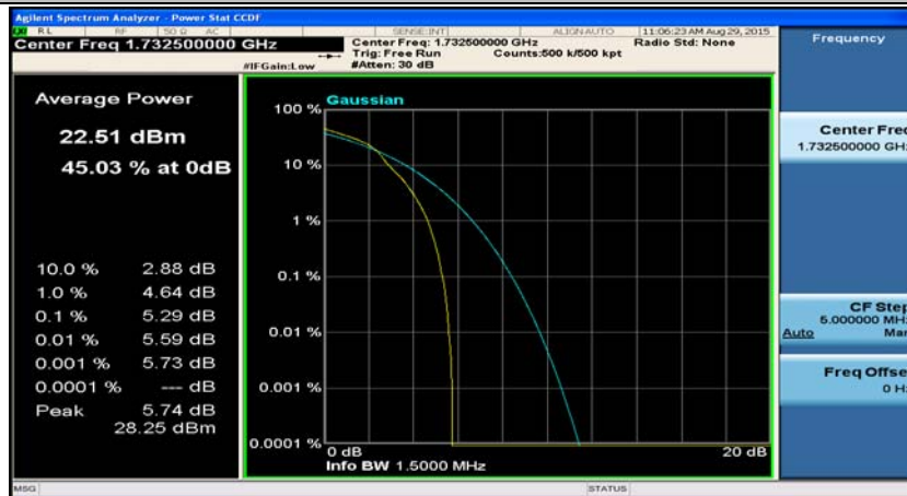
(Channel Bandwidth: 1.4 MHz)_MCH_16QAM_3RB#0
