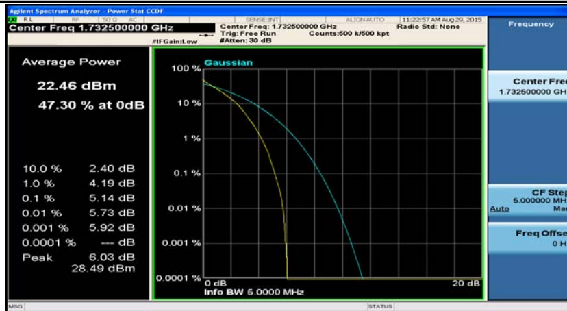
(Channel Bandwidth: 5 MHz)_MCH_QPSK_25RB#0
