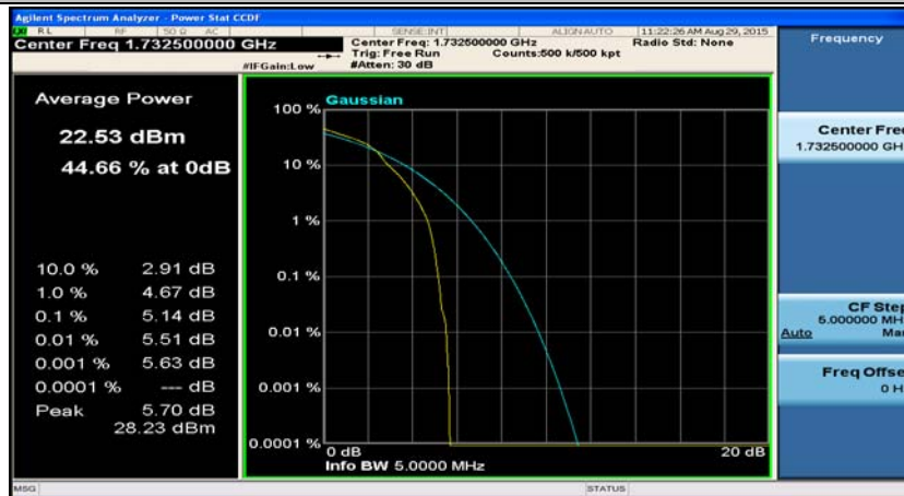
(Channel Bandwidth: 5 MHz)_MCH_16QAM_12RB#0
