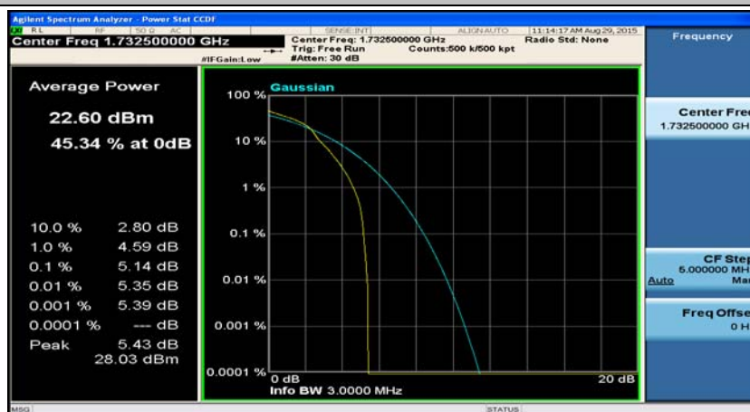
(Channel Bandwidth: 3 MHz)_MCH_16QAM_1RB#7
