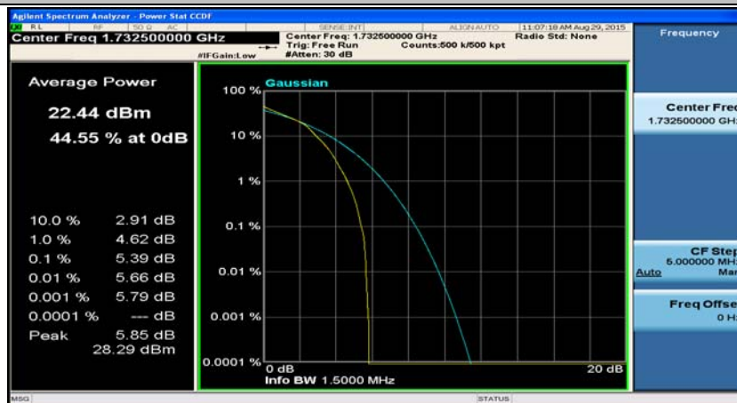
(Channel Bandwidth: 1.4 MHz)_MCH_16QAM_3RB#2
