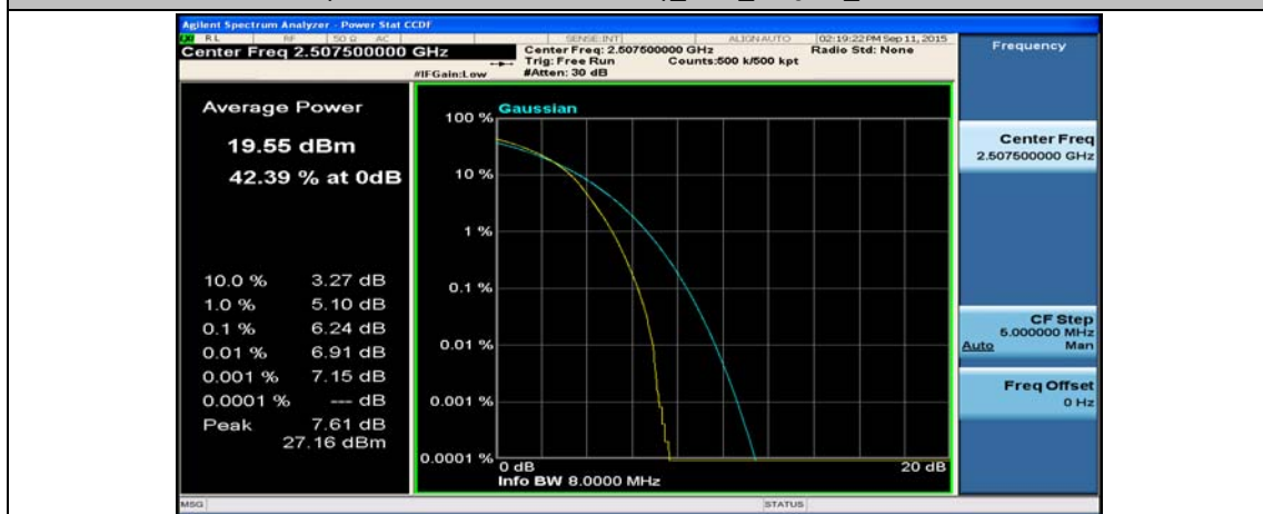
(Channel Bandwidth:15 MHz)_LCH_16QAM_75RB#0
