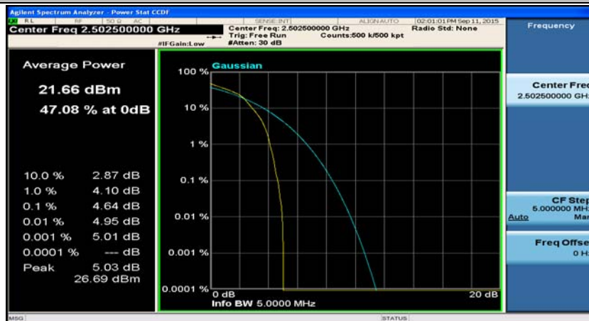
(Channel Bandwidth: 5 MHz)_LCH_16QAM_1RB#24
