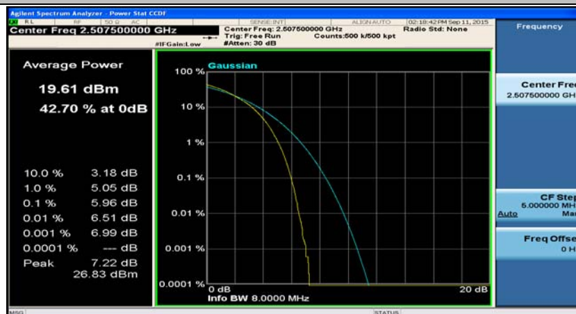
(Channel Bandwidth:15 MHz)_LCH_16QAM_37RB#38
