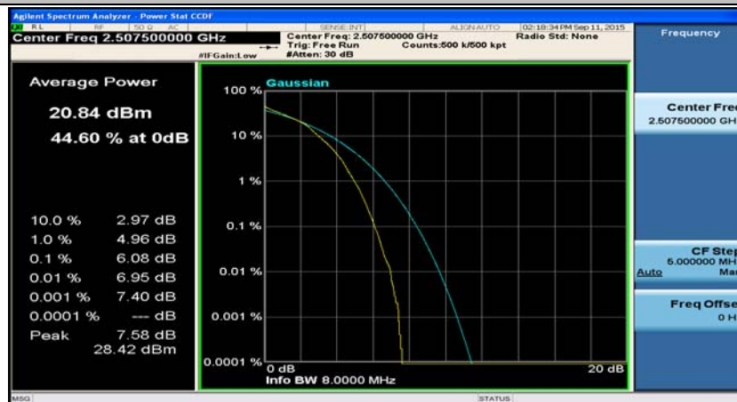
(Channel Bandwidth:15 MHz)_LCH_16QAM_37RB#38
