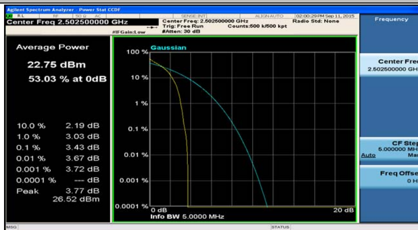
(Channel Bandwidth: 5 MHz)_LCH_QPSK_1RB#24
