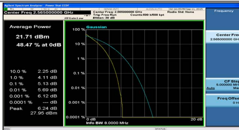
Channel Bandwidth: 10 MHz_HCH_QPSK_50RB#0
