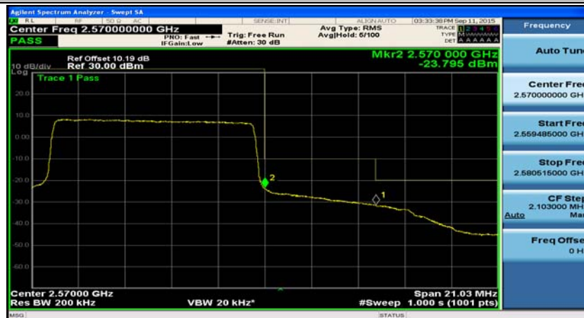
Channel Bandwidth: 10 MHz_HCH_QPSK_50RB#0
