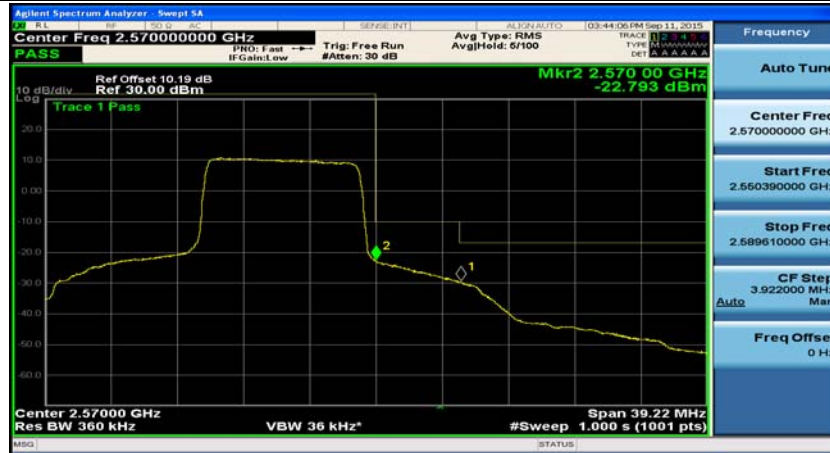
(Channel Bandwidth:20 MHz)_HCH_QPSK_100RB#0
