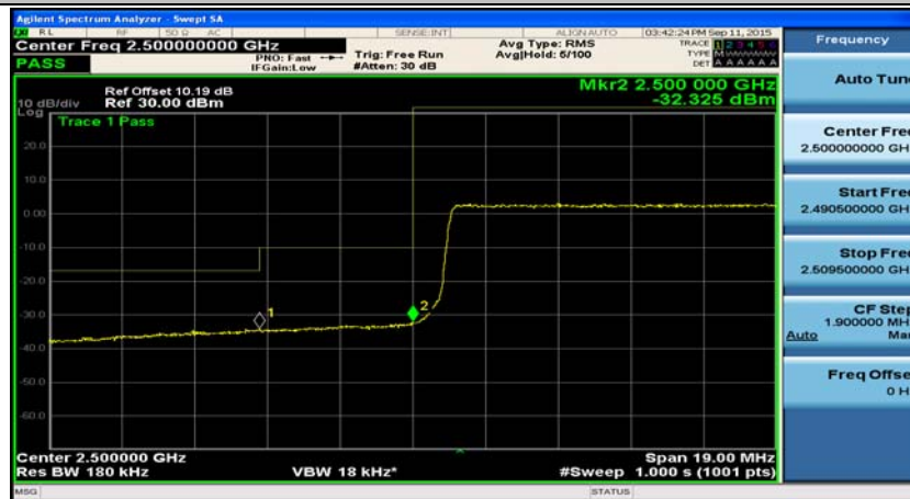
(Channel Bandwidth:20 MHz)_LCH_16QAM_100RB#0
