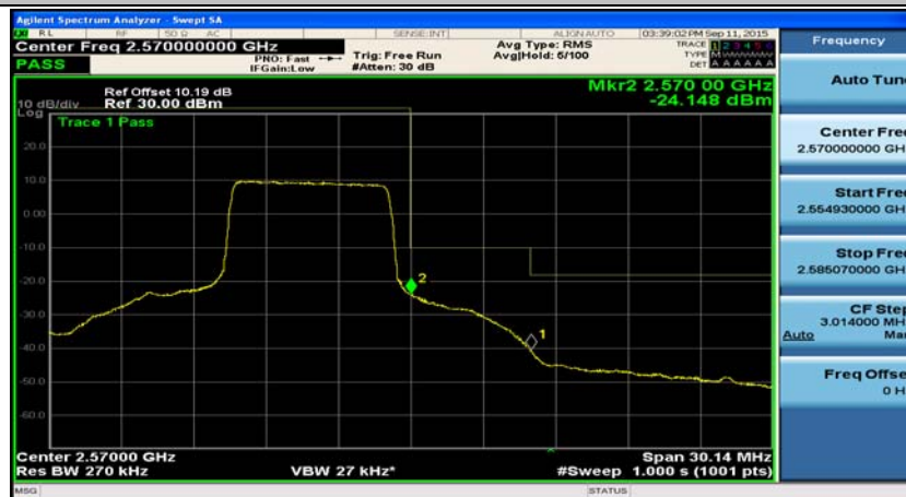
(Channel Bandwidth:15 MHz)_HCH_16QAM_75RB#0
