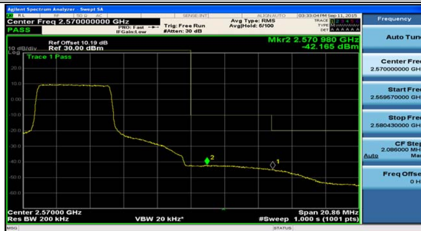
Channel Bandwidth: 10 MHz_HCH_16QAM_25RB#12
