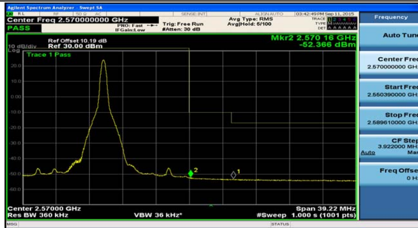
(Channel Bandwidth:20 MHz)_HCH_QPSK_1RB#49
