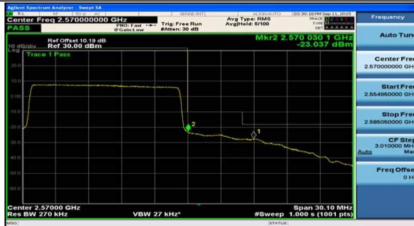
(Channel Bandwidth:15 MHz)_HCH_QPSK_75RB#0
