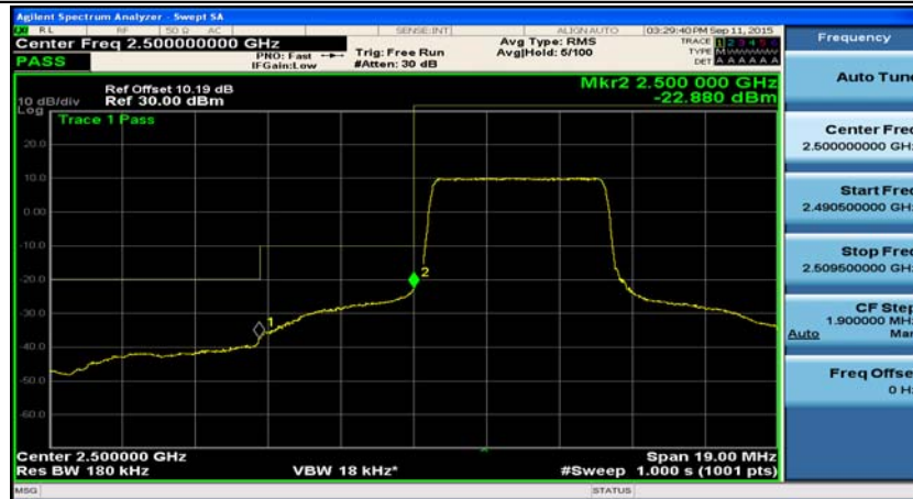
Channel Bandwidth: 10 MHz_LCH_QPSK_25RB#12
