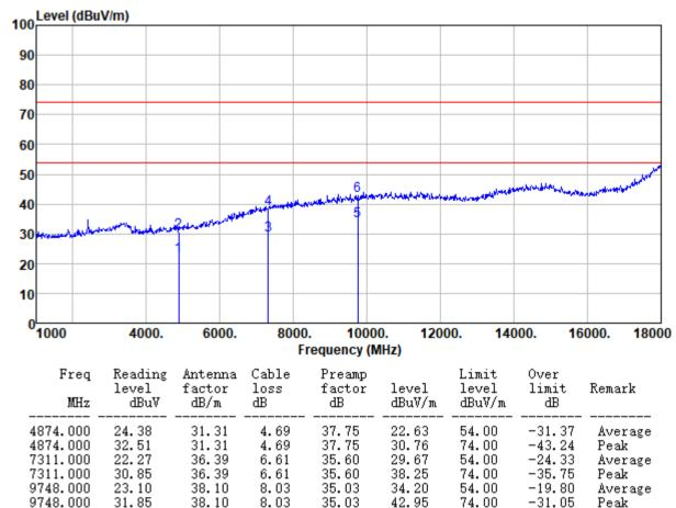
Remark: Final Level = Receiver Read level + Antenna Factor + Cable Loss - Preamplifier Factor
