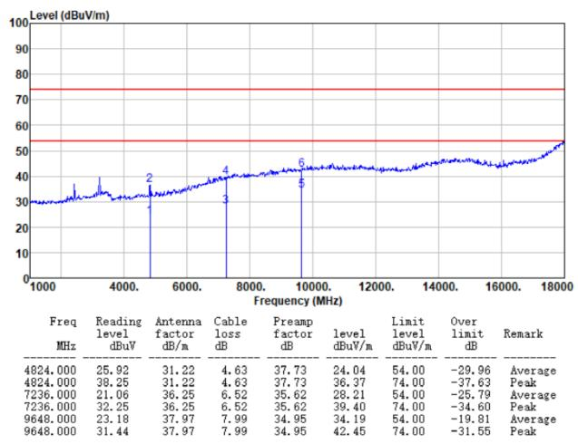
Remark: Final Level = Receiver Read level + Antenna Factor + Cable Loss - Preamplifier Factor
