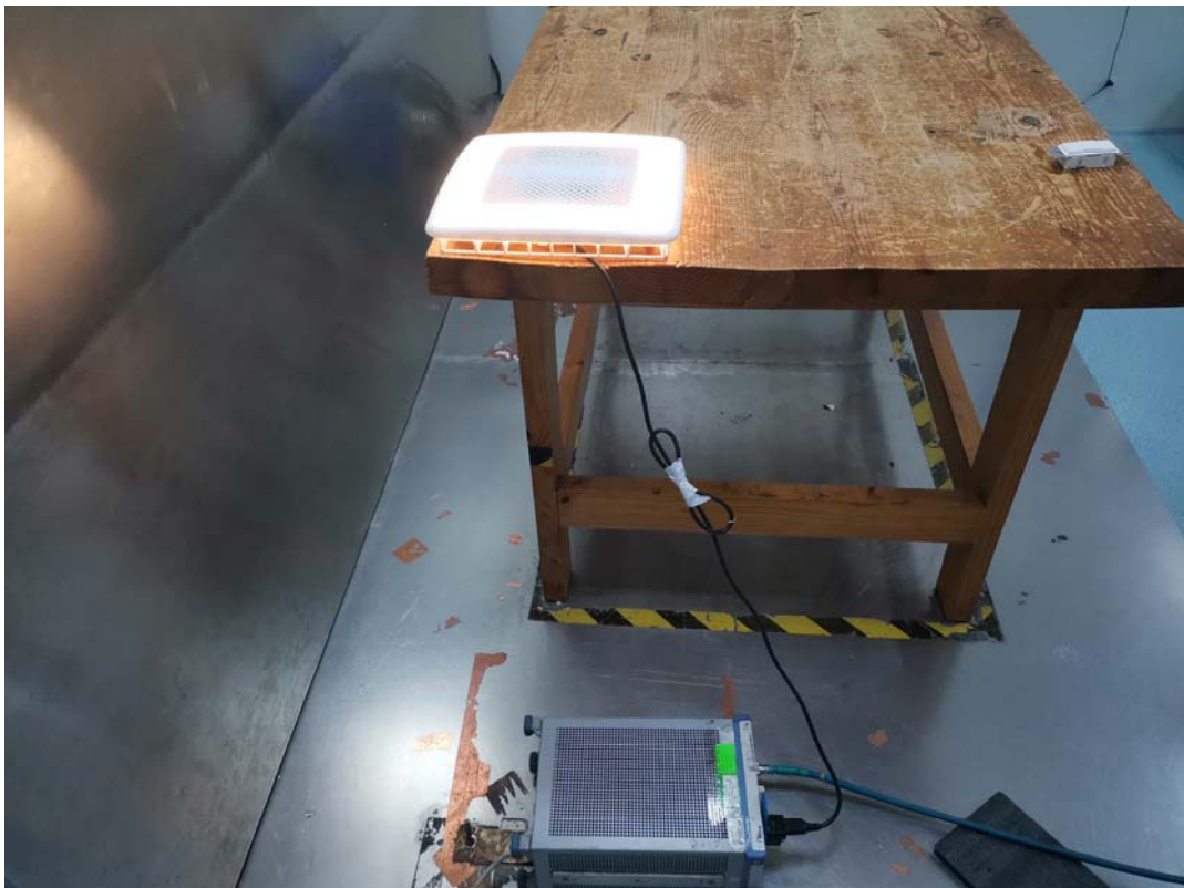
Conducted Emissions Side View
