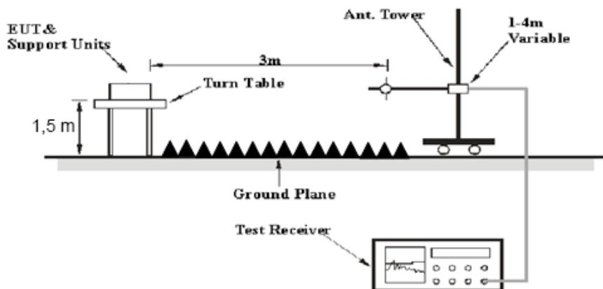
The radiated emission below 1GHz tests were performed in the 3 meters chamber test site A, above 1GHz tests were performed in the 3 meters chamber test site A, using the setup accordance with the ANSI C63.10-2013. The specification used was the FCC 15.209, and FCC 15.247 limits and the RSS-247 Clause 5.5, RSS-GEN Clause 8.10 limits.
