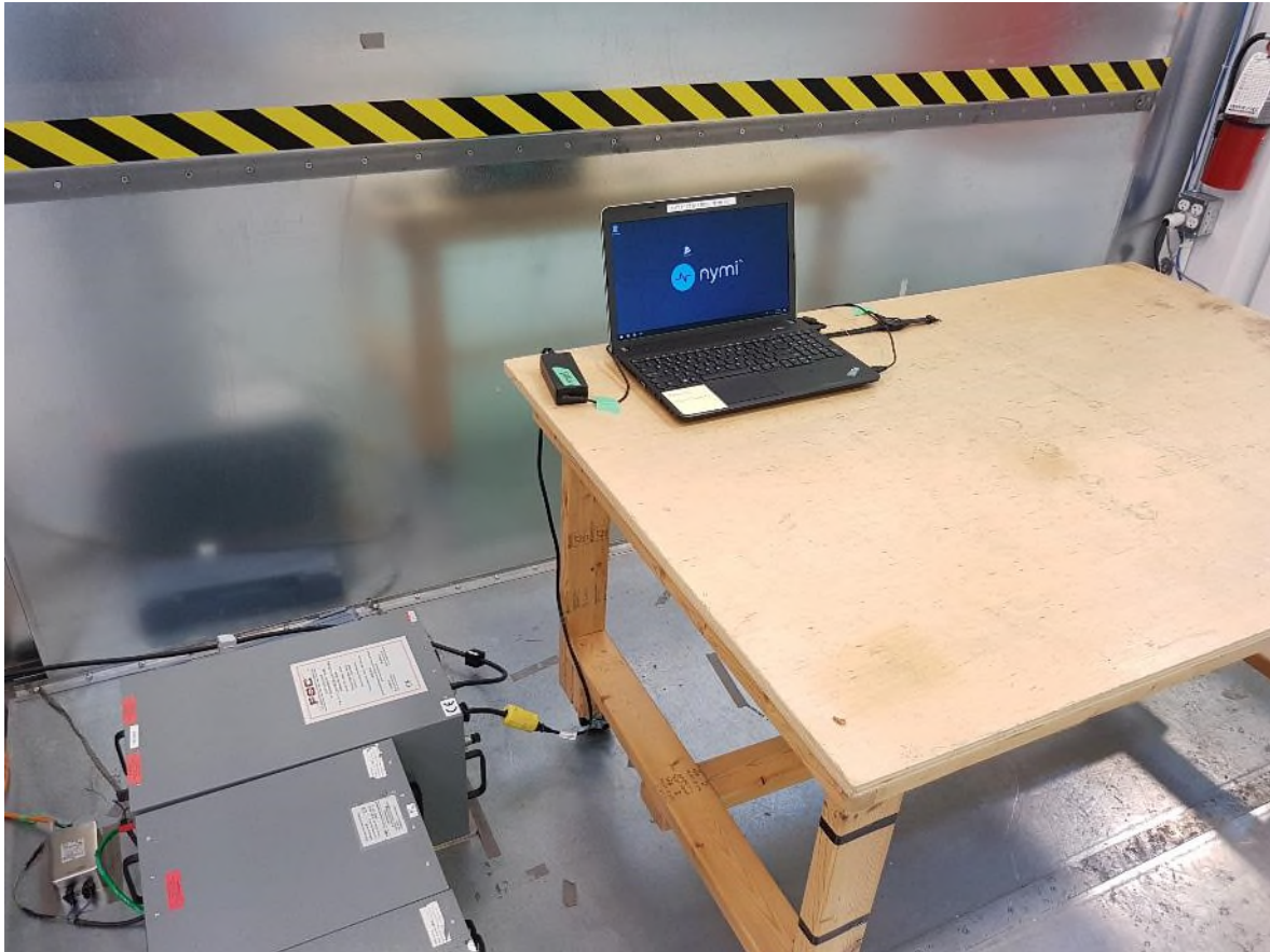
Figure 7 – Conducted Emissions Setup
