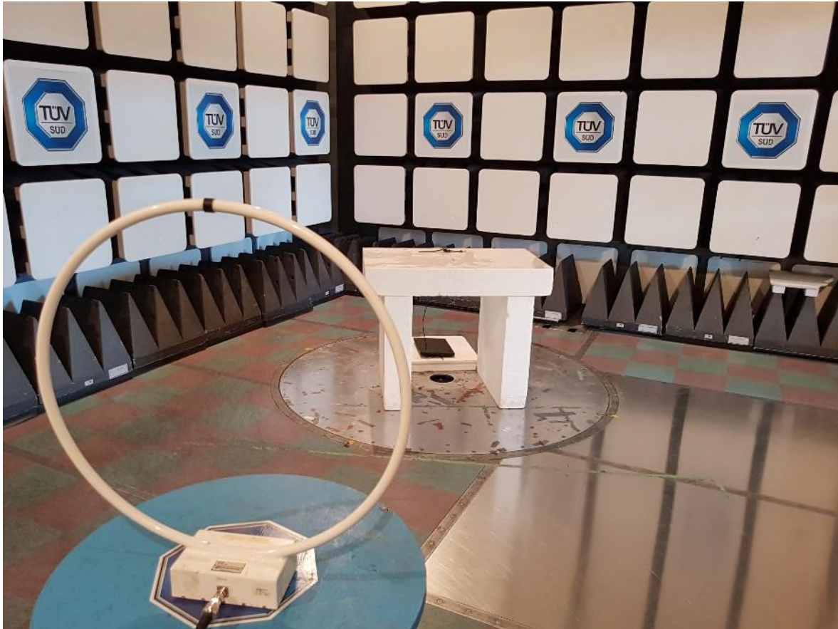
Figure 3 – Radiated Emissions Setup
