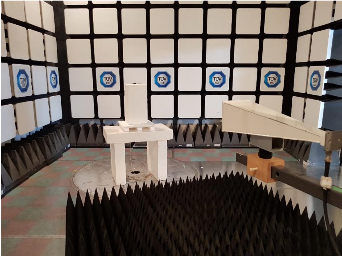
Figure 5 – Radiated Emissions Setup
