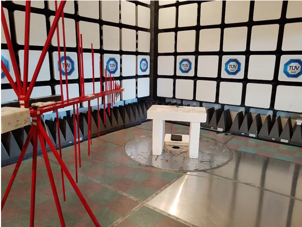
Figure 4 – Radiated Emissions Setup
