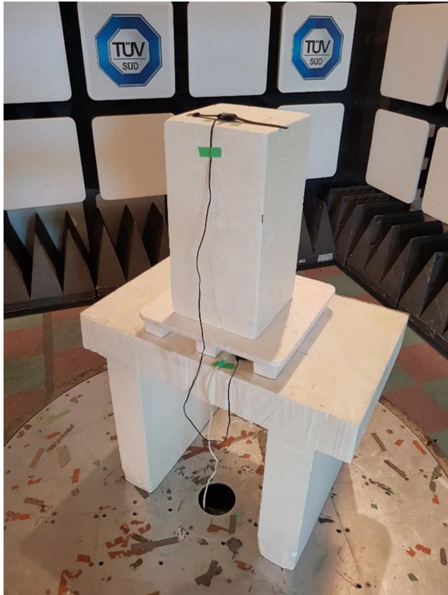
Figure 2 – Radiated Emissions Setup
