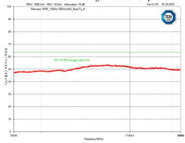
Plots were taken at a 1 meter distance. All emissions were noise floor of measurement instrument. No emissions were found in this frequency range.
