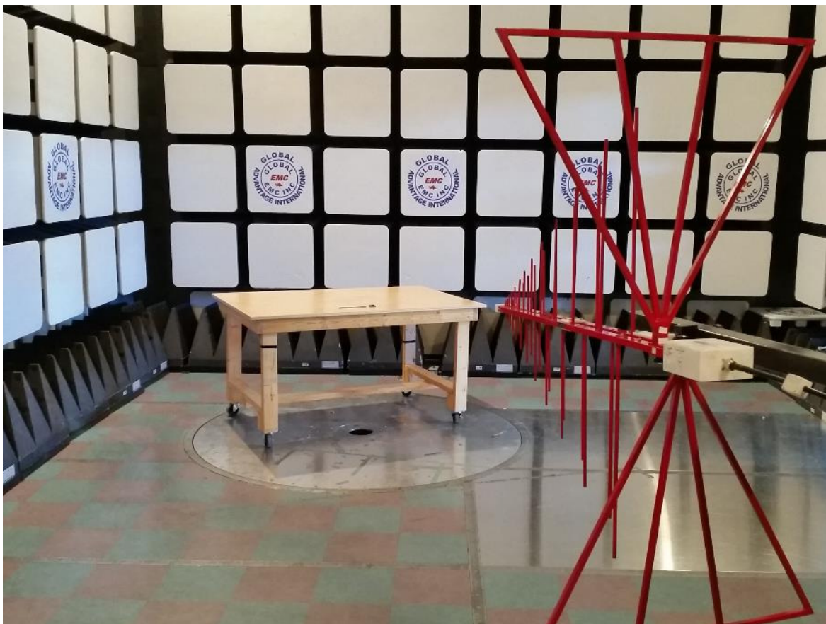
Figure 3 – Radiated Emissions Setup – Photo 2
