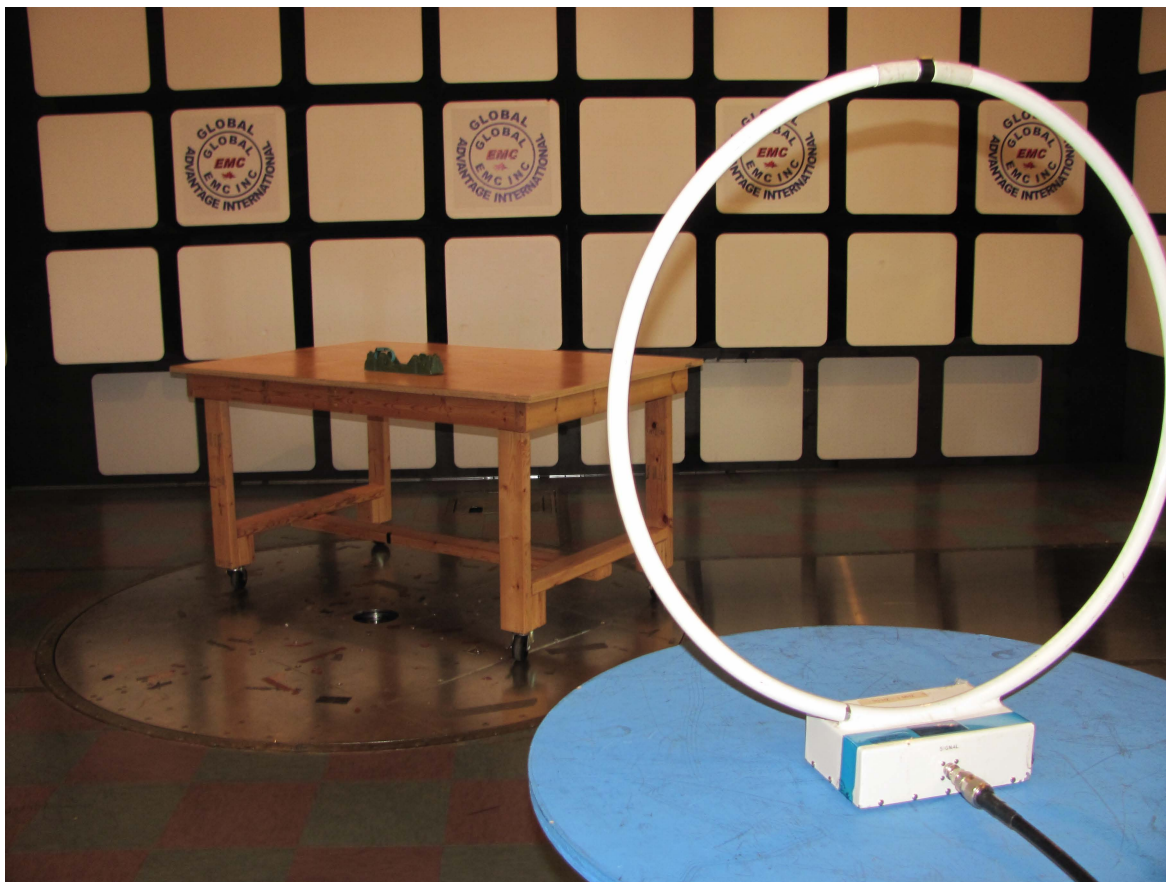
Illustration 1: Radiated emission setup – photo 1
