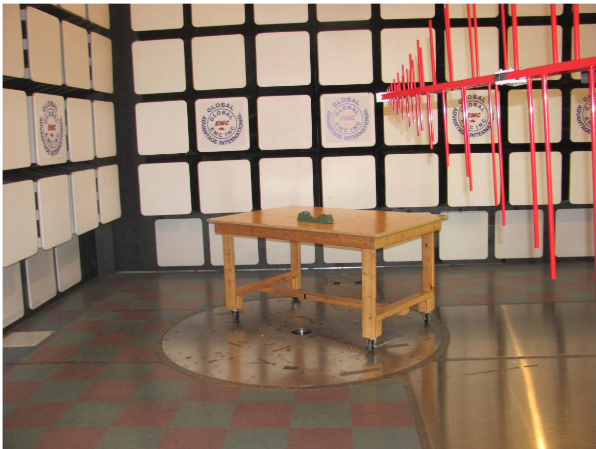
Illustration 2: Radiated emission setup - photo 2
