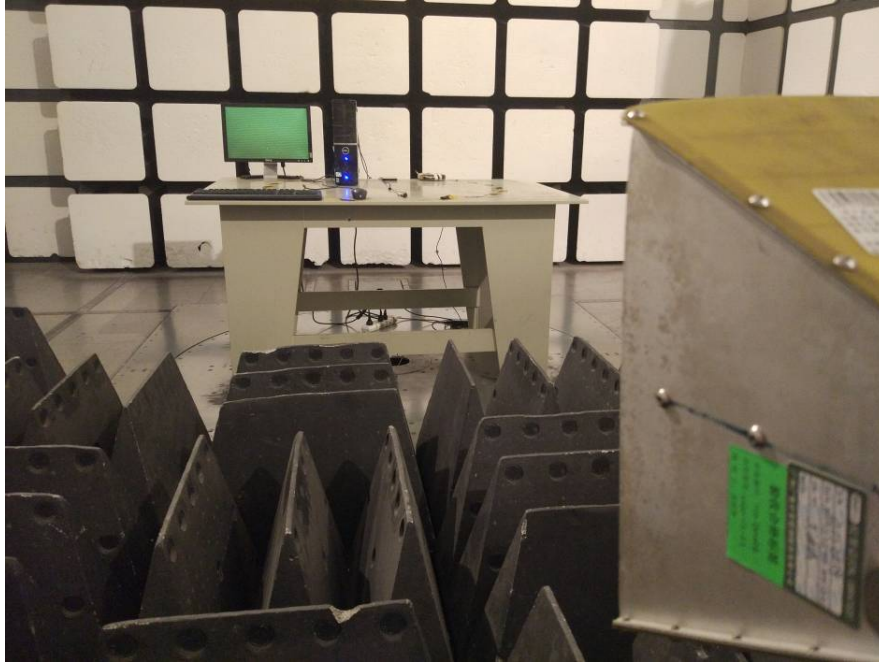
Radiated Emissions – Front View (Above 1 GHz)
