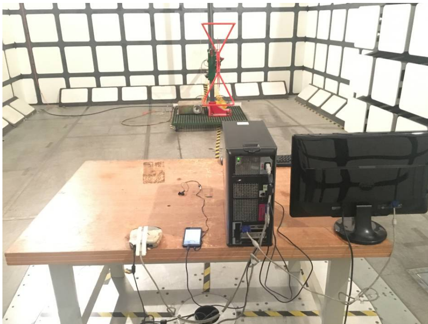
Radiated Emissions – Rear View (Below 1 GHz)
