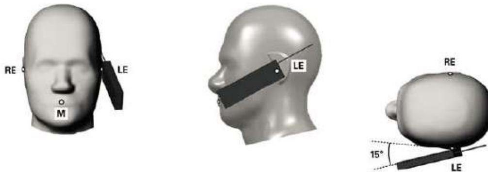
Fig.11.4 Illustration for Tilted Position
