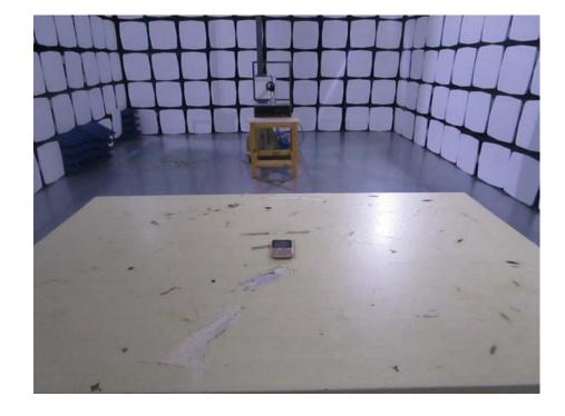
Spurious Radiation Test Setup (9kHz to 30MHz)
