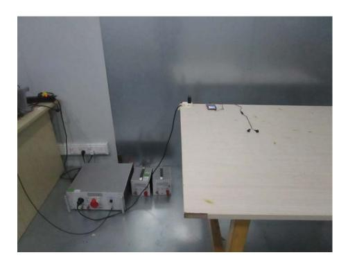
Radiation Emission Test Setup (Below 30MHz)
