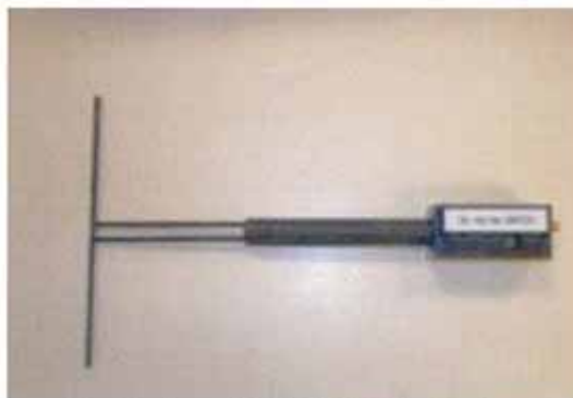
Figure 1 – Satimo COMOSAR Validation Dipole
