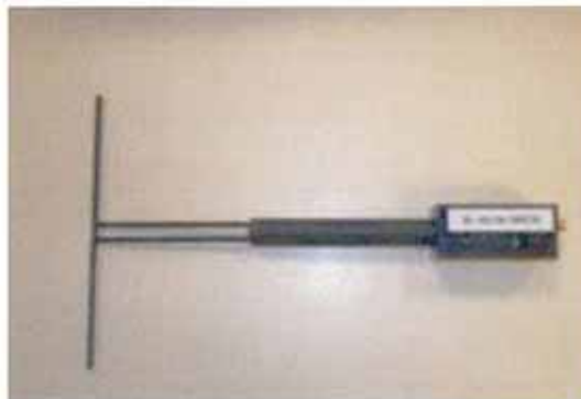
Figure 1 – Satimo COMOSAR Validation Dipole
