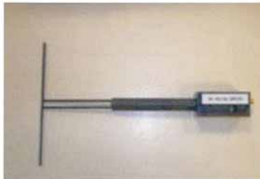
Figure 1 – Satimo COMOSAR Validation Dipole
