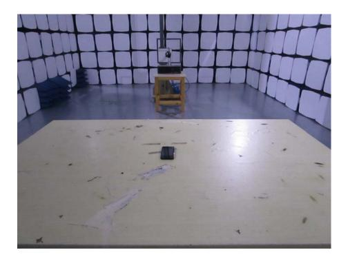
Spurious Radiation Test Setup (30MHz to 1G)
