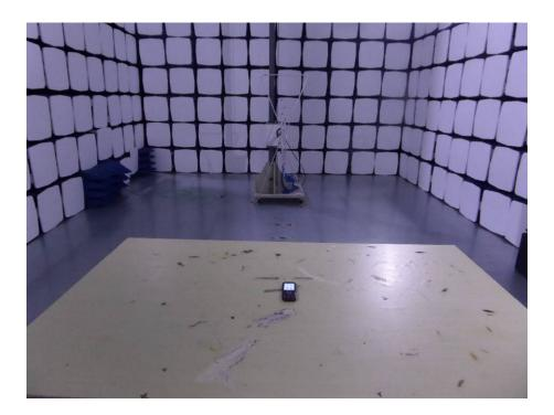
Radiation Emission Test Setup (Above 1GHz)
