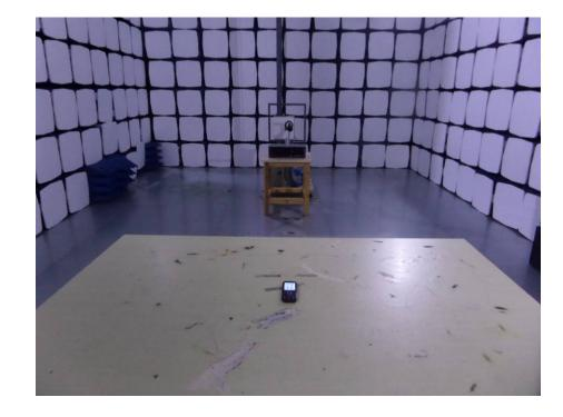
Spurious Radiation Test Setup (9kHz to 30MHz)
