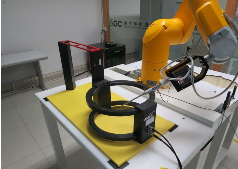
T-Coil setup with HAC Test Arch and AMCC
