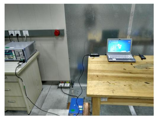
FCC RADIATED EMISSION TEST SETUP
