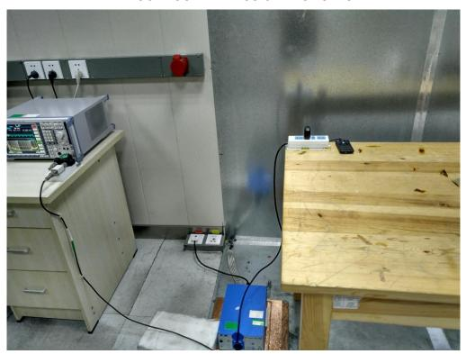
RADIATED EMISSION TEST SETUP
