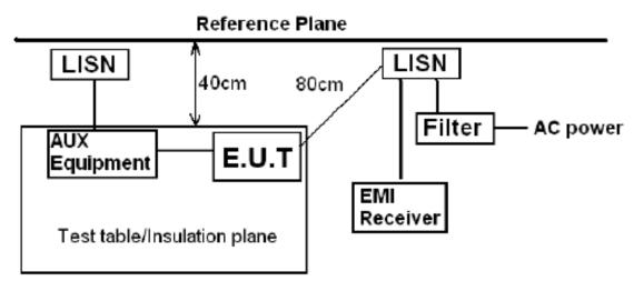
Remark E.U.T: Equipment Under Test LISN: Line Impedence Stabilization Network Test table height=0.8m
