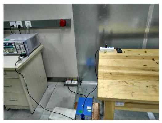
RADIATED EMISSION TEST SETUP
