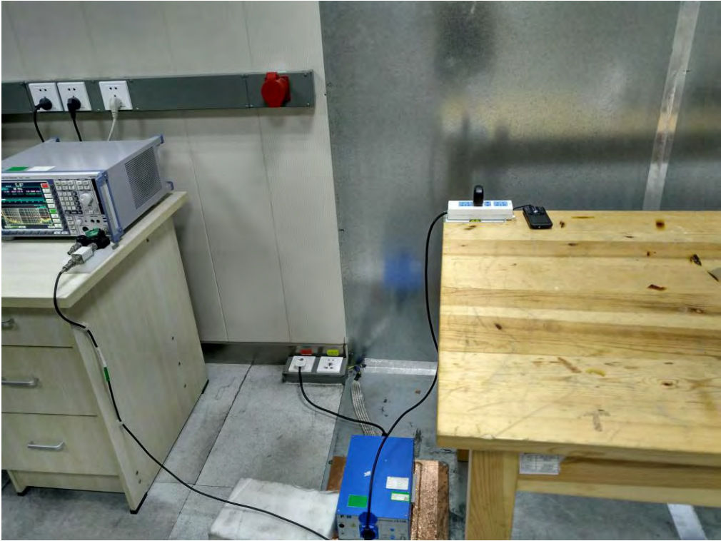
FCC RADIATED EMISSION TEST SETUP
