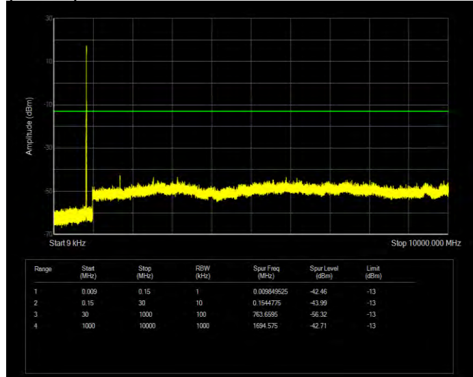
Band26(824-849) 16QAM BW=5MHz Channel=26815 RB Size=25 Position=#0
