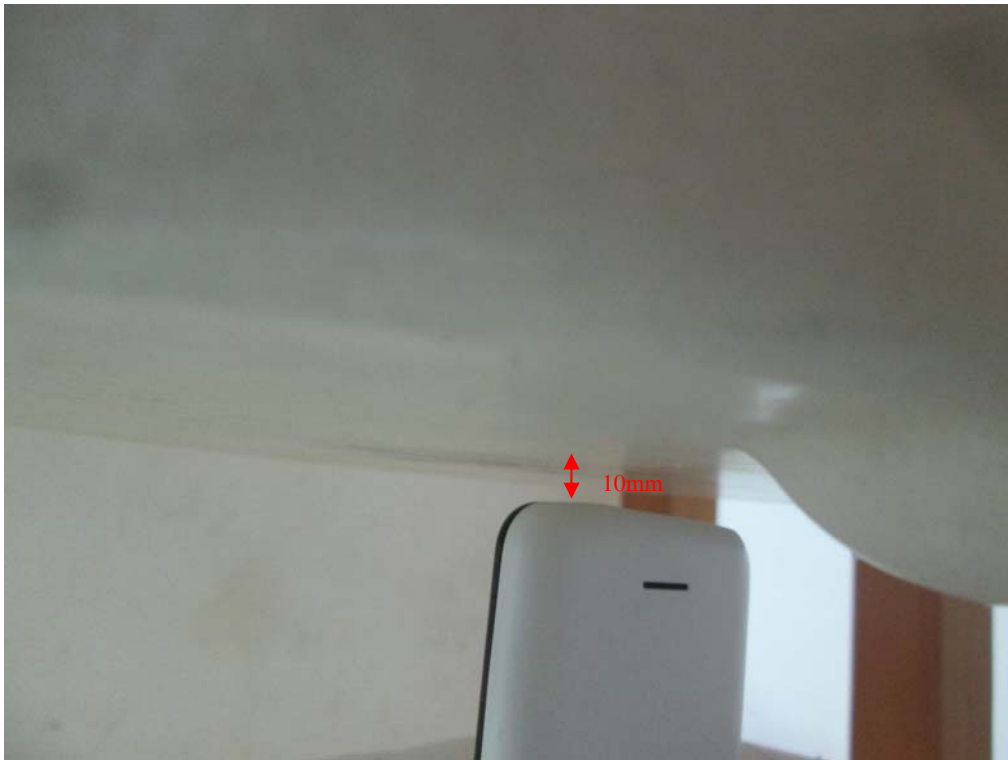
Body-worn Bottom Setup Photo (10 mm)
